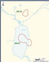
Figure 3: Model 2 is one large pipe based on ground geophysical surveys and limited core drilling. The apparent irregular pipe shape was suggested to be similar to southern-African kimberlites (Table 1).
